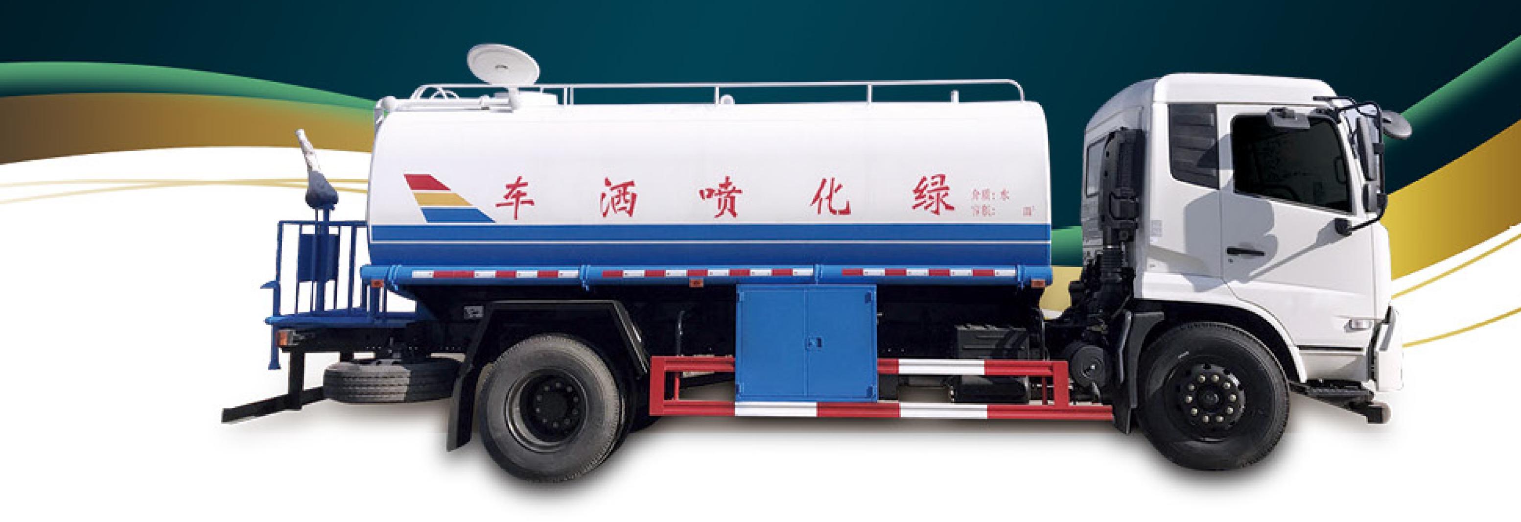
Sprinkler is suitable for all kinds of road washing, trees, green belts, lawn greening, roads, factories and mining enterprises construction construction, high-altitude building washing. It has the functions of water sprinkling, dust suppression, high and low level spraying, pesticide spraying, guardrail washing, etc. It also has the functions of water transport, drainage and emergency fire-fighting.
